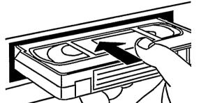
Insert the cassette into the cassette slot with the label facing towards you. The window must be facing upwards.
